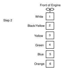
Write the corresponding colour of each cylinder next to your coil number on the lines marked X on the drawing. This will ensure that the sequence of spark is correct.
